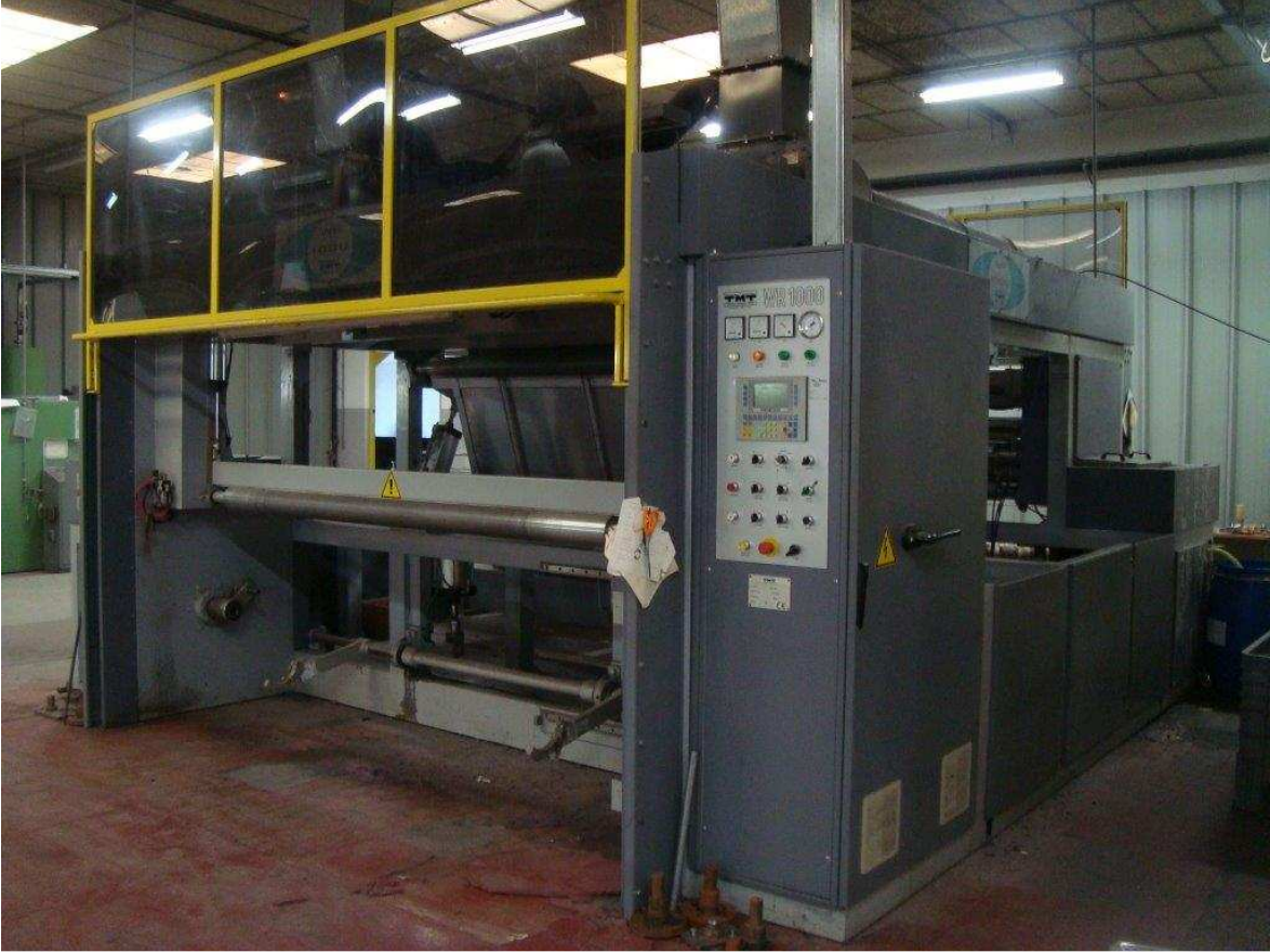
N°1 TMT SIZING MACHINE WR 1000 W:2500 YOC 1997 (CE) TANGENTIAL MODEL,AND OVEN WITH INFRARED HEATERS
